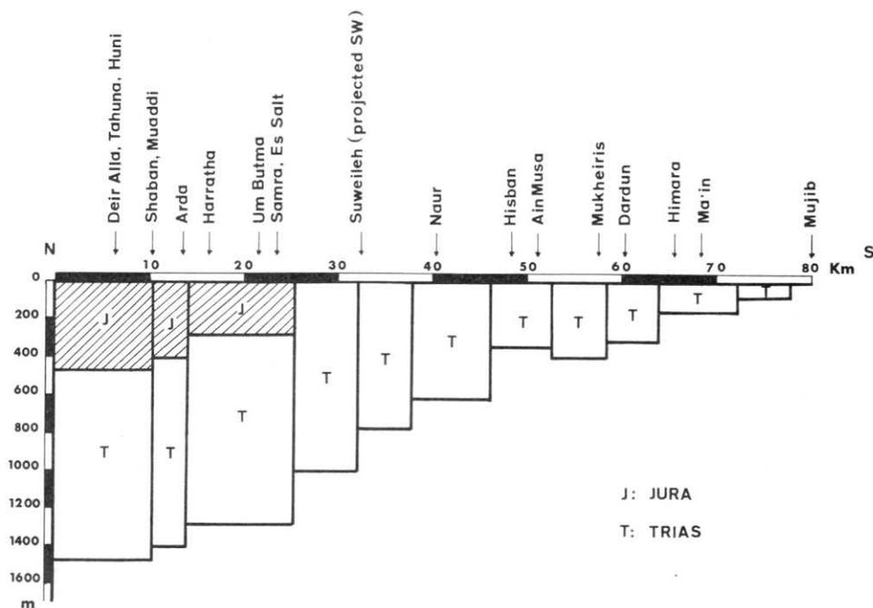
Fig. 12. Scetch demonstrating the step faulted, peneplained surface of the eroded Mesozoic rock column as it had been before deposition of the Lower Cretaceous Kurnub sandstones between the mouth of the river Zarqa (N) and the mouth of the Mujib river (S).
